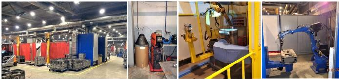
The "Welding" working unit has 44 cabins for welding and assembly of boilers. Welding machines "Kemppi" contain WiseFusion software that optimizes the welding parameters, central supply with Krysal mixture of gases (Ar+CO2), welding wire is distributed in 250 kg barrels in all workplaces, welding masks with adjustable photo-gray protection glass, usage of electric forklifters, ...finally, working in these conditions is a real pleasure.
