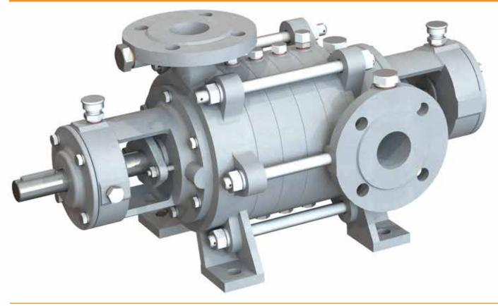
The C type range is the basic range of our centrifugal ring section multistage pumps. The simplified design, utilizing hydraulically balanced impellers by means of holes into impeller, or by "back to back" impeller execution, provides the optimum pumping solution for medium pressure applications. Pump casing is consisted of suction and discharge housing, middle chambers and bearing brackets. All of the impellers are centrifugal of closed type, and are statically and dynamically balanced.
