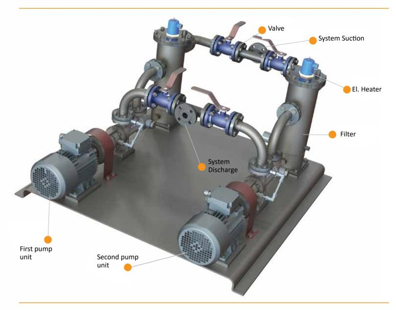
System SVPF os a system of two or three screw pumps of which one is duty and one is stand by, connected with suction main pipe with filter before each pump and discharge main pipe. The whole system is mounted on one steel base frame equipped with anchor bolts and ready for concreting.
