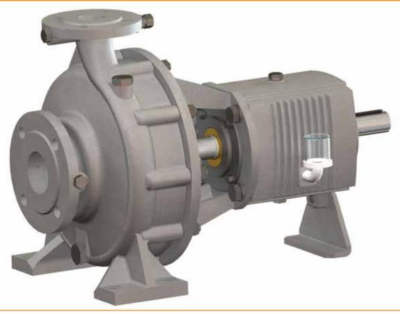
Single stage, low pressure, centrifugal end suction pump with an axial inlet into the impeller and flanged bearing frame. Simple and compact design, suitable for flexible coupling to electric motor or internal combustion engine as a drive. Fast and easy dismantling without detaching from the existing pipeline.
