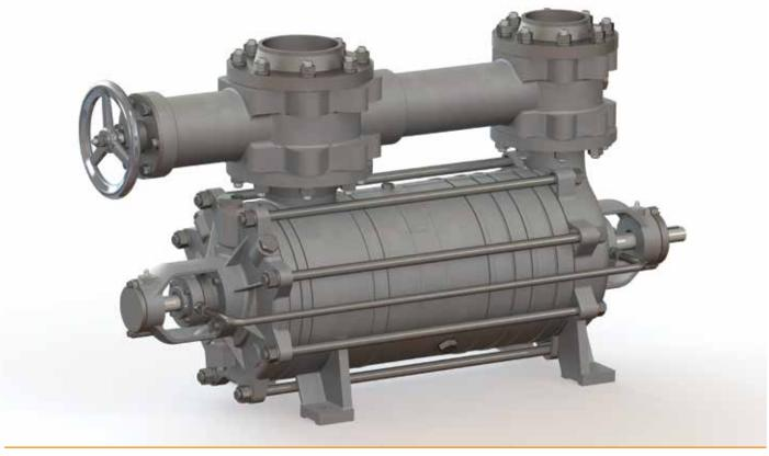
BCP petrol pumps are centrifugal, self-priming, horizontal pumps. They are assigned for transport of all kinds of petrol and diesel. They also could be used for transport of ammonia, benzol etc. BCP pumps are designed as single stage and multistage. They can be driven by electric drive on the same base plate. Self-priming of the pump is made possible by means of the vacuum rotor which is enclosed in the pump.
