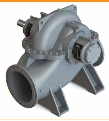
Horizontal Split Case Double Suction Centrifugal Pumps Type: D are engineered to pump clean water or low viscosity clean liquids at moderate heads more efficiently than any other type of pump. All fabricated parts are standardized and accurately machined for true alignment, increasing overall durability. Impellers are statically and dynamically balanced and constructed with double inlets, practically eliminating the axial thrust and resulting in high operating efficiency.
