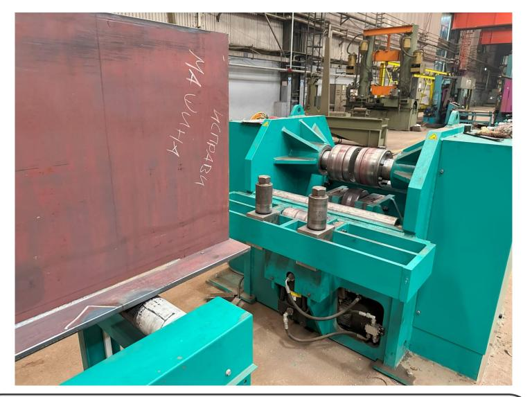
Type: Welded sections streightening Manufacturer: Stierli-Bieger, Switzerland Pressing force: 500 kN Flange dimensions (W x T): 150 – 800 mm (H-beam) ; 100 – 400 mm (T-beam) x 5 – 20 mm Web dimensions (H x T): 250 – 2000 mm x 4-20 mm Length: 1500 – 15000 mm
