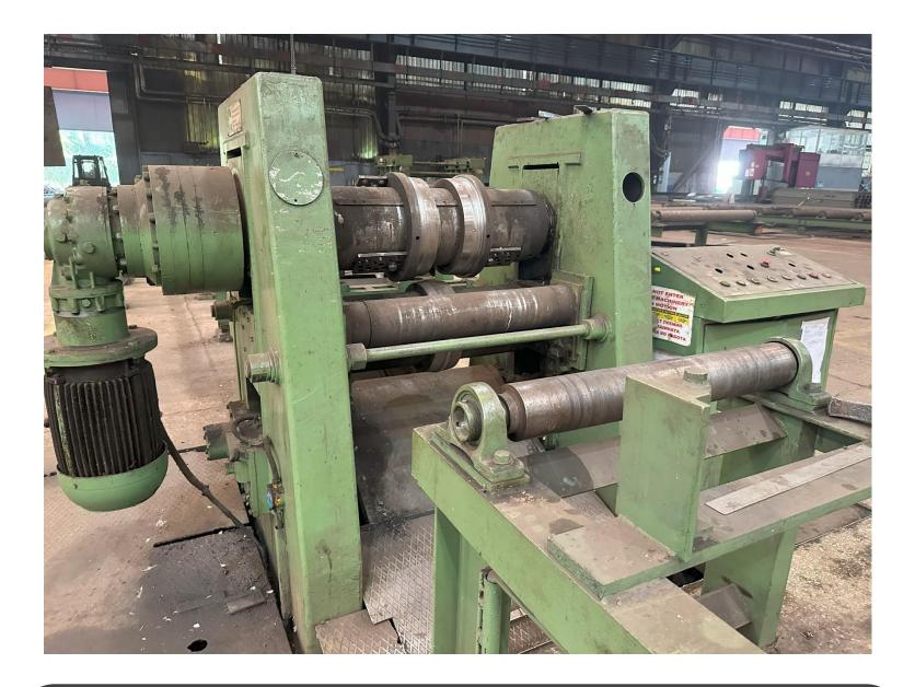
Type: Predeformation- plate prestressing (IP 700x35) Manufacturer: Di Parmigiari, Italy Max. plate width: 700 mm Max. plate thickness: 35 mm Speed: 14 m/min
