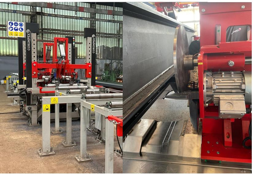
Type: Edge rounding machine Manufacturer: CORIMPEX, Italy Flange width: 160-1250 mm Web thickness: 6 - 25 mm Working speed: 2.5 - 3 m/min
