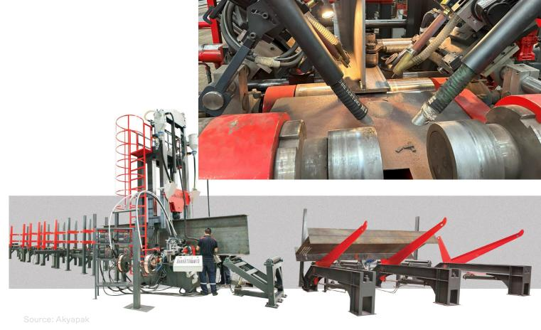
**Type:** Automatic SAW welding machine (HBW 2000x1000) Manufacturer: Akyapak, Turkiye Beam types: H, I, T, L with 4 torches Beam width: 150 - 1000 mm Beam height: 200 - 3500 mm Flange/ web thicknesses: 8-60 mm / 6 – 40 mm
