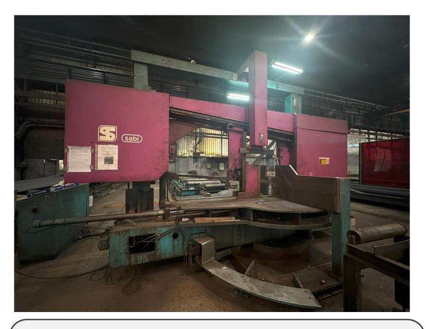
Type: Beam saw Manufacturer: SABI, Spain Max. dimensions: 1350 x 600 mm Max. plate thickness: 35 mm Angle cutting: -60 to +45 degrees
