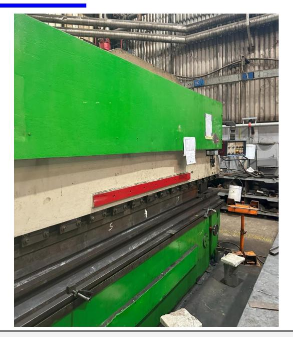
Type: Press brake (PI 175) Manufacturer: SIMEROM, Romania Max. plate length: 4050 mm Max. plate thickness: 8 mm
