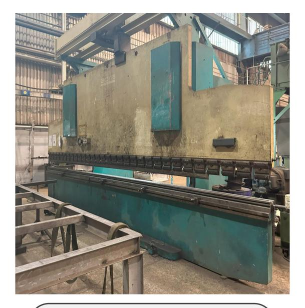
Type: Press brake (QHD-20040/60) Manufacturer: ADIRA, Portugal Maximum capacity: 2000kN Max. working length: 6.1 m Stroke: max- 200 mm; min- 15 mm Max. working speed: 7.9 mm/s
