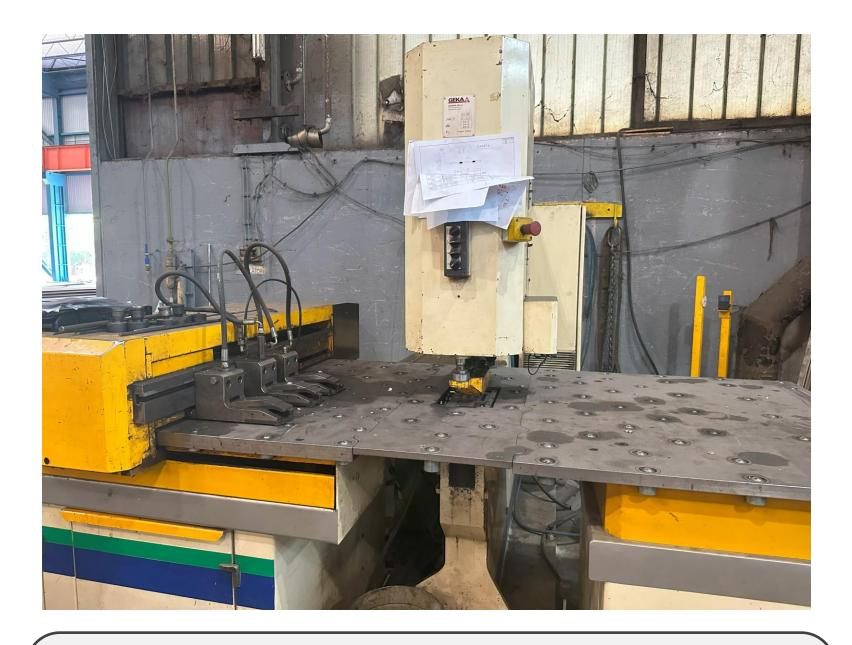
Type: CNC Punching (PAXY 1500, PUMA 110) Manufacturer: GEKA, Spain Workspace: 750 x 1515 mm Max. thickness: 28 mm (diameter 28 mm)
