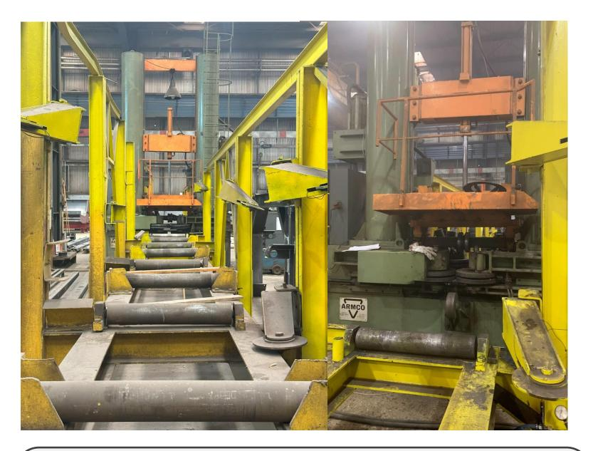
Type: Arc welding machines Manufacturer: ARMCO, Italy Number of lines: 12 Beam dimensions: 700/200/3000 mm Welding sources: Lincoln Electric DC-1500 A
