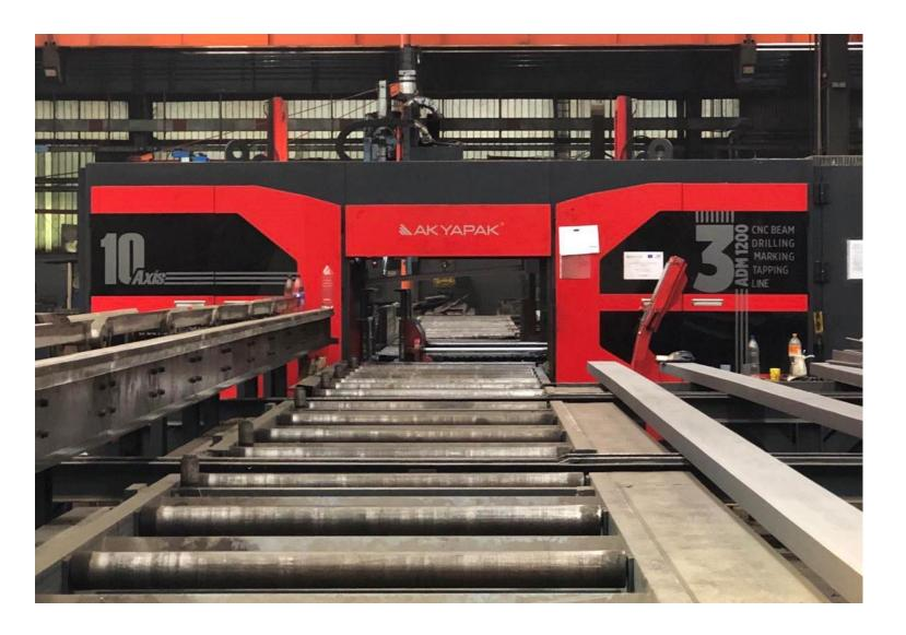
Type: CNC beam saw (AST 130 - 600) Manufacturer: Akyapak, Turkiye Sawing capacity max. (W x H): 1300 x 600 mm Sawing capacity min. (W x H): 65 x 45 mm Cutting speed: 20 - 100 m/min Type: CNC beam processing (3 ADM 1200) Manufacturer: Akyapak, Turkiye Max. beam dimensions (H x W): 500 x 1200 mm Drilling diameter: 10 – 40 mm Weight per linear meter: 750 kg/m
