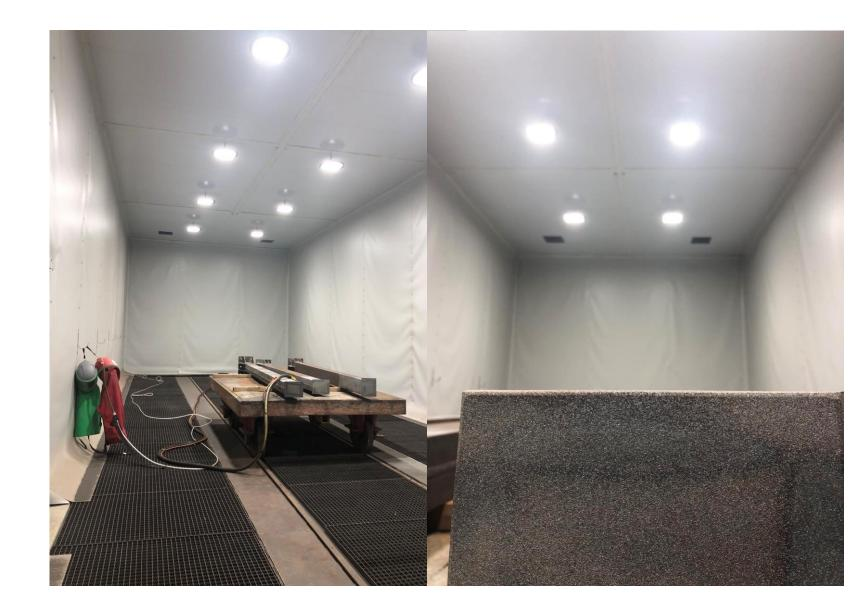
Type: Manual sandblasting equipment (293.K) Manufacturer: Tovarna industriske opreme, Slovenia Number: 2 Work pressure: 10.4 Pa Capacity: 0.015 m<sup>3</sup>
