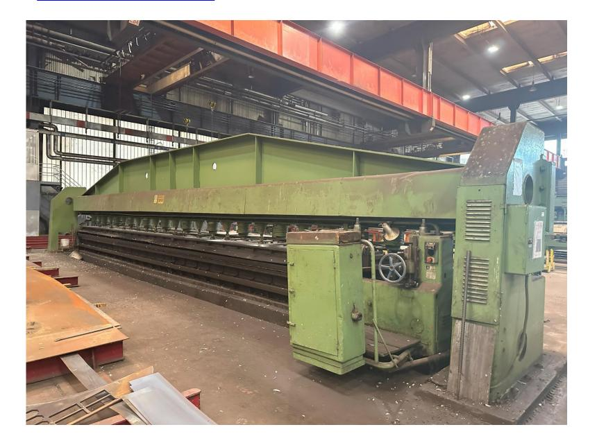
Type: Plate bevelling machine Manufacturer: HULIN TOS, Czechoslovakia Max. plate length: 14 m Max. plate thickness: 80 mm Max. speed: 12 m/min
