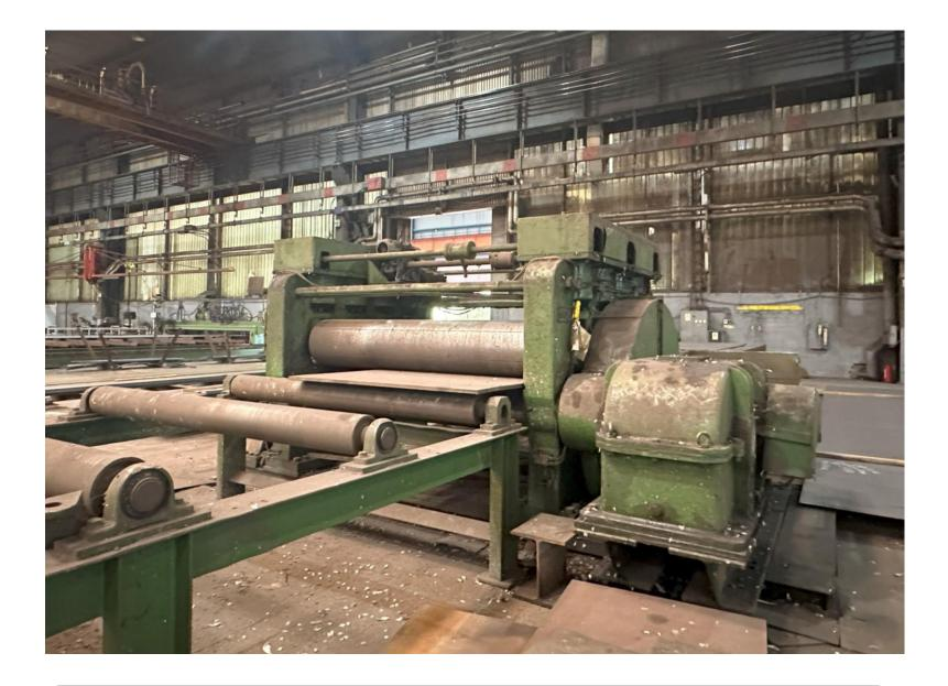
Type: Predeformation- plate straightening Manufacturer: Di Parmigiari, Italy Max. plate width: 2000 mm Max. plate thickness: 30 mm
