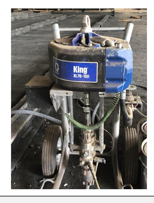
**Type:** Shotblasting hall **Manufacturer:** SAPI, Germany **Dimensions (L x W x H):** 16 x 6 x 5 m Type: Manual painting equipment (XL 70-180) Manufacturer: GRACO, USA Max. fluid WPR: 500 bar Max. air WPR: 7 bar
