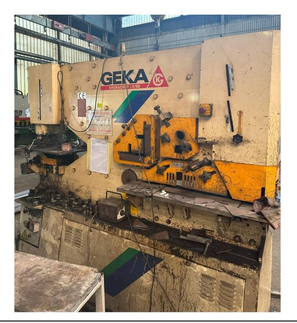
**Type:** Drilling and cutting (HYD 110) **Manufacturer:** GEKA, Spain **Max. diameter:** 40 mm **Max. plate thickness:** 35 mm **Max. hole diameter:** M 16
