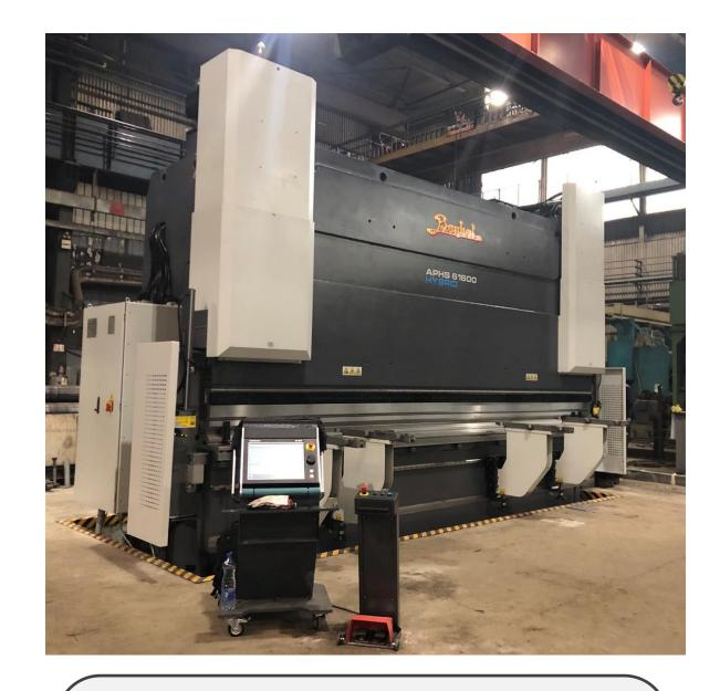
**Type:** Press brake (APHS HYBRID 61600) Manufacturer: Baykal, Turkey Bending force: 600 t Max. bending length: 6.1 m Stroke: 625 mm **CNC** controller
